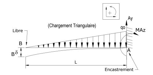
$$\delta_B = \frac{qo \times L^4}{30EI} = \frac{10 \times 10^{-3} \times 2,70^4}{30 \times 2.1 \times 10^{+5} \times 1000 \times 10^{-8}} = 8,43.10^{-3} m = 8,43 mm$$
