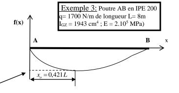
$$pour x = 0.421L \approx 3,37m \Leftrightarrow y_{\text{max}} \approx \frac{-1700 \times 10^{-3} \times 8000^{4}}{185 \times 200000 \times 1943 \times 10^{+4}} = -9,68mm$$
